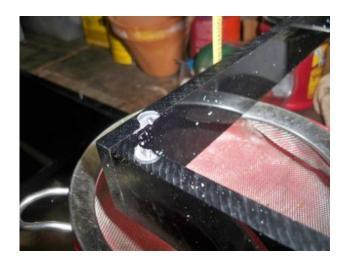
prepare the brackets that will hold the glass in place. At the corners of the main body, on only one side (which will become the lower side) use a Forstner bit in a drill press to drill out some
