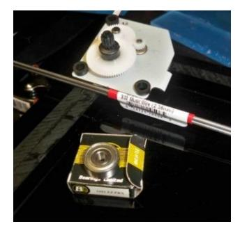
The radial bearing with the smallest center hole was still larger than the rod, just under 1/16" inner diameter. I very slightly tapered the end of a 1/16" brass rod to fit into the bearing, and used a drill press to drill out a 3/32" hole in the exact center. The necessary piece of brass (now a hollow cylindrical adapter sleeve) was cut off and used to attach the drive belt gear to the radial bearing.
