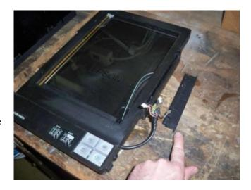
The only other things holding the two parts of the body together are two plastic taps on the side of the body opposite the two screws. If you're careful you may be able to separate the halves without breaking them. I was not.
