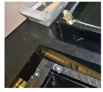
This is close-up of a corner of the base after drilling gaps to receive the screw heads. Note also how the pieces come together to increase strength.
