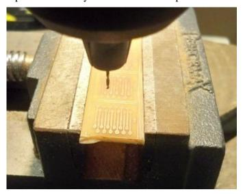
The individual boards will look like this. Four of these are necessary to connect 6 FFC into two 4 foot cables. You may want to use 3 18" cables as some of the length will be used up inside the scanner head, making the connection.
