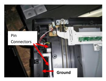
A small flat-head screwdriver can be used to carefully pry the pin connectors loose. If you don't want to lose screws, put them back in place right away, starting with the ground wire screw.
