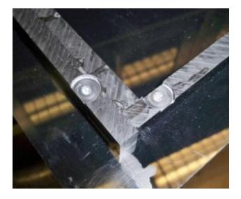
This image shows the finished side brackets holding the glass in place from the bottom (upper), and the corresponding gaps in the base (lower) for the screw heads.
