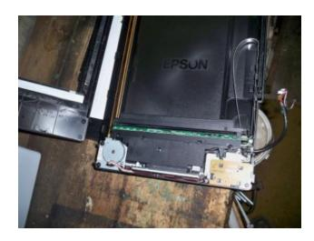
We will replace this metal bar with one much longer. First we need to get a very precise diameter measurement. You can remove the drive belt by unscrewing the gear housing at the far end, but be careful to note how it is threaded through all the gears and tensioner first.
