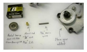
Here is the gear, radial bearing, brass sleeve, and wire rod assembled and ready to insert into the scanner. I will drill out an appropriately sized hole in the supports later to hold the bearing steady and thus take the sideways strain of the drive belt.
