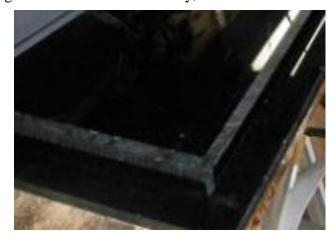
I also used a double wall in the base design at both ends to add some additional strength. This may not be necessary with plastic this thick, but it will keep those joints bombproof, and create a very strong base to build upon.
