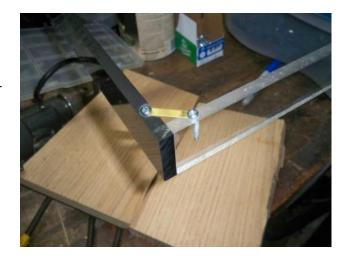
Line up the holes needed and drill them out. Doing this one bracket at a time and cutting the piece off at the final end after drilling will keep the pieces manageable and safer to drill. Drill through into block of plywood or hardwood to reduce deformation. Round off the corners by filing or snipping.
