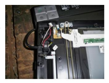
Have a quick look at the mechanism used to move the scanner head. There is a stepper motor running the gears. This is similar to what we will face in the main body of the scanner as well. One challenge is going to be to find a belt the correct size.
