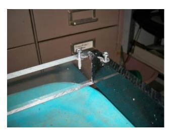
Drill or route out a 12" or so channel in the middle of the two long sides of the main body to hold metal glass supports. I made these from the inner wall to about ¾ of the way to the outer wall. These and the previous round pits near the corners are all about 1/32" deep, just enough to offset the metal brackets. Drill 4 holes spaced along the removed channel in the middle of the plastic wall. Tap them as with the corner bracket holes.
