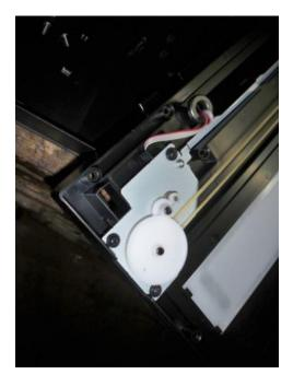
At any time, you can remove the hinge from the lid by extending it all the way out, opening the lid all the way, and pressing the lid and body towards each other. There are two screws holding the body together. Once these are undone you can pry the body apart a bit and slide the hinge out.
