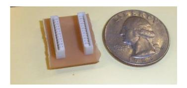
Use electrical or other tape to ensure the cable connections are not strained by being pulled at a tight angle at the connector during use. If there is insufficient room along the side of the scanner as it goes by for this, you will need to carefully kink the FFC at 90 degrees.
