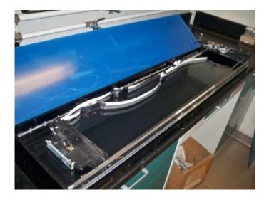
You can simplify some of the layout of individual parts by salvaging the ends of the original scanner case. I saved both ends by cutting them out with a hacksaw. Note the motor and gear assembly is not in position in this photograph; it is simply sitting loose.
