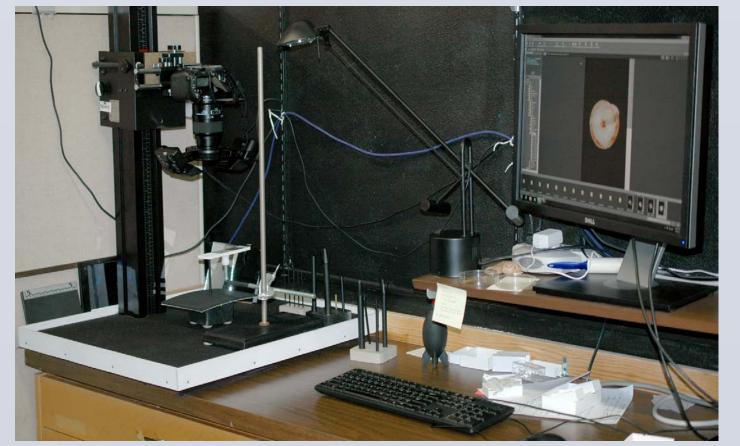
**Z-stacking rig,** for specimens 2.0-5.0 mm. Automated computer-controlled Z-stacking; manual lighting
