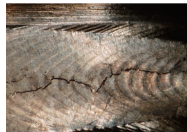
Section Fatigue Crack (50x)
