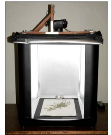
Figure 2. Front side of the Lightbox with the front panel removed, a custom specimen holder inside, and a custom camera mount.
